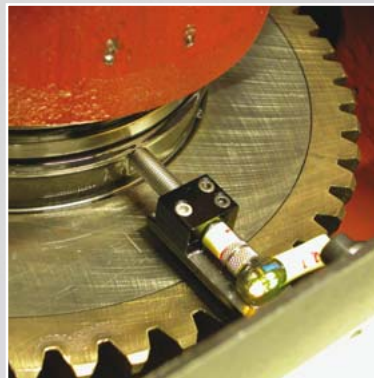
■ Detail of 4 independent overload release clutches
